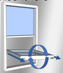
Grip the sides of the sash and with even pressure rotate one side up and one side down allowing sash to be removed from frame.
