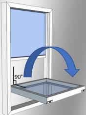
On top of sash squeeze tilt latches inward toward center.
