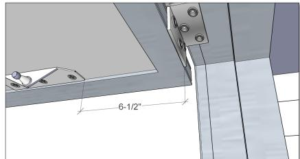
Install second gas prop bracket 6-1/2" from top of door frame with ball stud facing the center of the door/awning. Do not mount bracket on extrusion.
