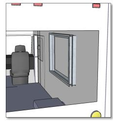
Step 2 Once your door/awning is firmly secure remove shipping clips and install gas prop brackets. First install one bracket on your door/awning's frame 19-3/4" down from inside of top of the frame. Ball stud should be facing outward.
